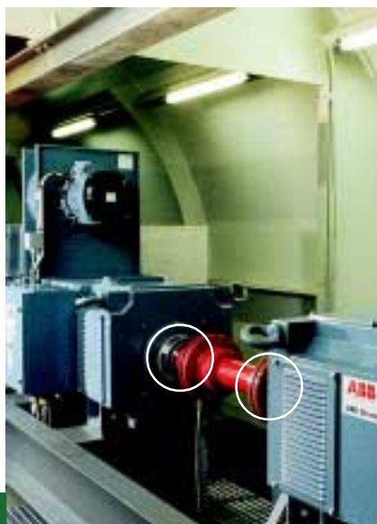
Figure 25: Digital-Tachos HG 18 without bearings synchronize two DC gear motors coupled by a cardan shaft.
