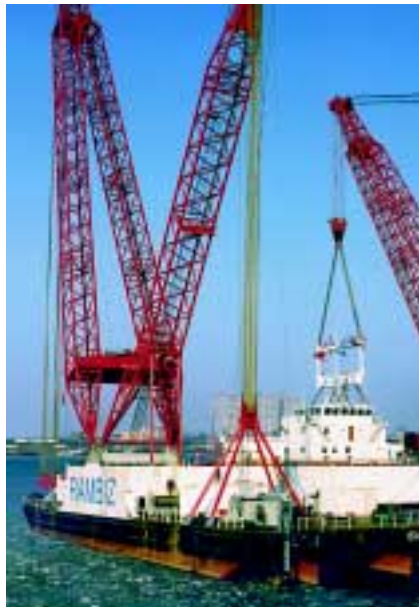
Sea air and ice, heat and moisture – all the extreme weather that this planet can produce: the hoist and boom drives on this 2 x 2,000 t crane ship are fitted with HOG 10 and POG 10 Digital-Tachos from HÜBNER.
