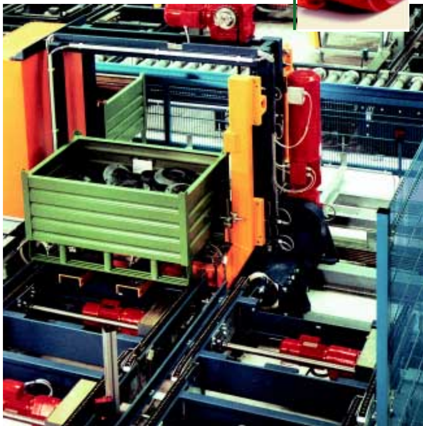
Automatic guided vehicles steer precisely to their destination: HÜBNER HOG 71 Digital-Tachos measure the speed of the networked gear motors.
