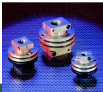
Figure 27: HÜBNER spring disk couplings with insulated hub protect against shaft currents.
