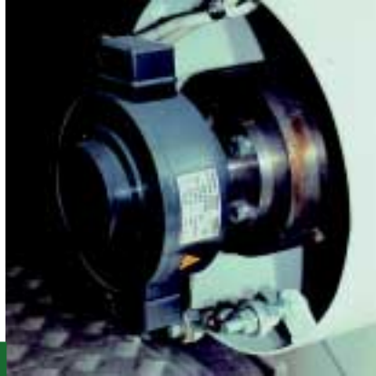
Figure 5: Redundant scanning, the HOG 16 on a 2,600 kW drive as example.
