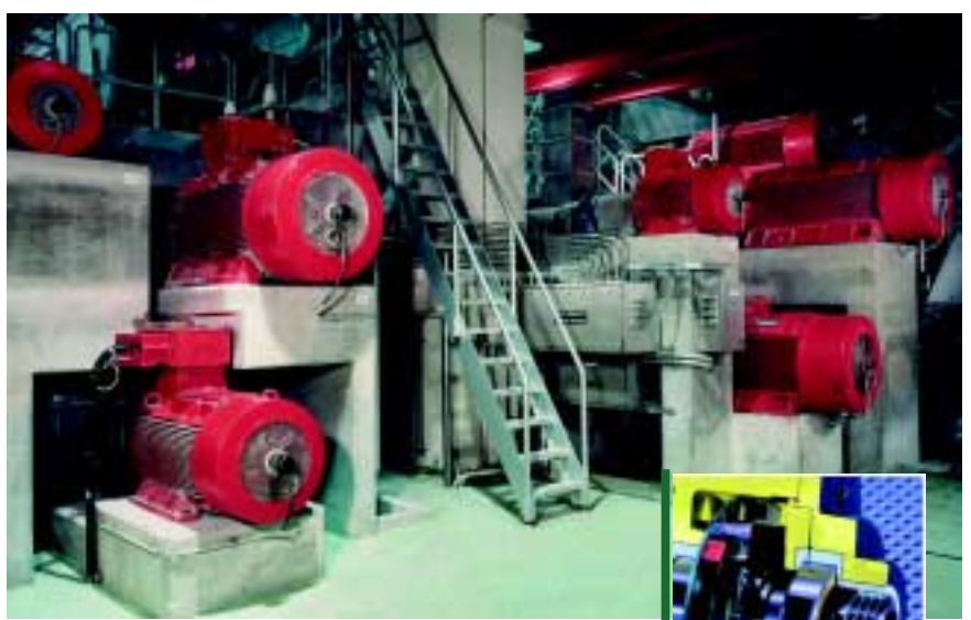
Highest reliability in continuous operation: HÜBNER HOG 10 Digital-Tachos, with insulated bearings for protection against shaft currents, synchronize the drives on this paper machine, and on many other similar plants, „round the clock“.
