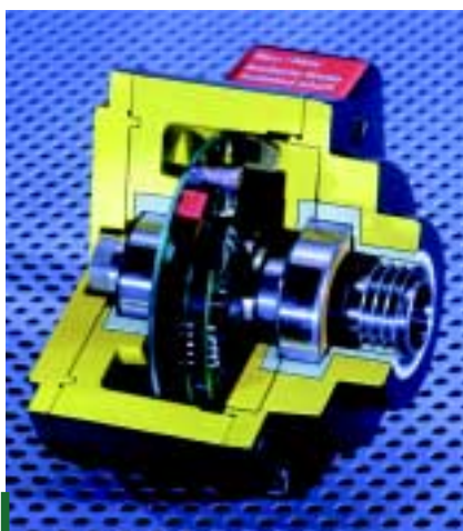
Figure 22: HeavyDuty® technology in top form: solid alloy housing, generously sized, insulated ball bearings, scanning electronics with power transistors mounted between the bearings, labyrinth seal for protection class IP 66 (HOG 10).
