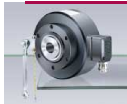
Fig. 14: Combination of Digital-Tacho + earthing contact to ground shaft currents (HOG 16).
