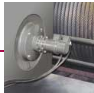
Fig. 3: Twin-Encoder with two different values of pulses per turn, on a 450 kW drive (POG 9 G).
