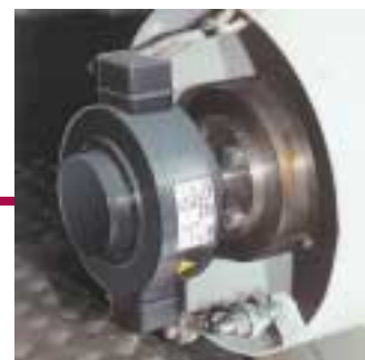
Fig. 4: Redundant sensing of the incremental disk, in this case on a 2,600 kW drive (HOG 16).
