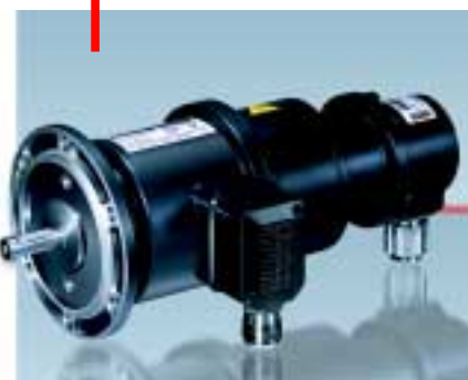
Figure 30: The rear shaft of the Analog-Tacho drives via a coupling within a rear support housing the Digital-Tacho with own bearings (TDP 0,2 + OG 60 or separate encoder).
