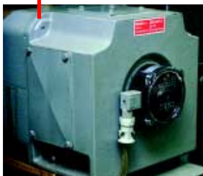
Figure 12: Hollow-shaft tachogenerator (GTB 9 in IP 68) on a precision CNC machine.
