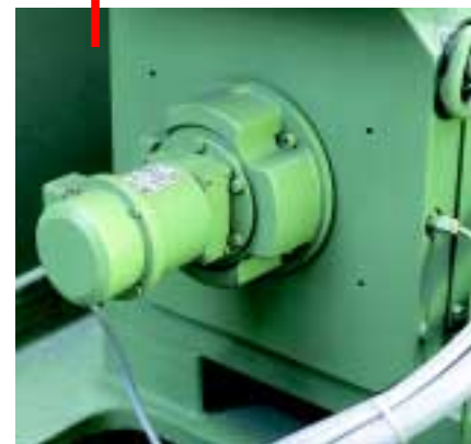
Figure 27: Twin tachogenerator with two winding system (TDPZ 0,2) – here on a drive of a cold forming press.
