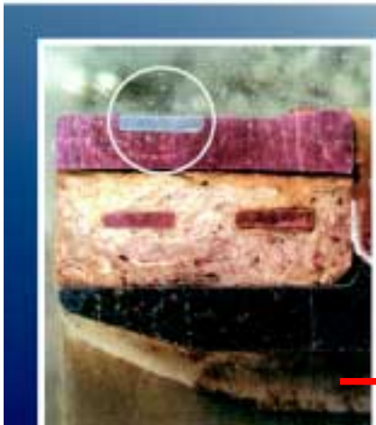
Figure 7: Hollow-shaft armature (GTB 9) with embedded silver track.
