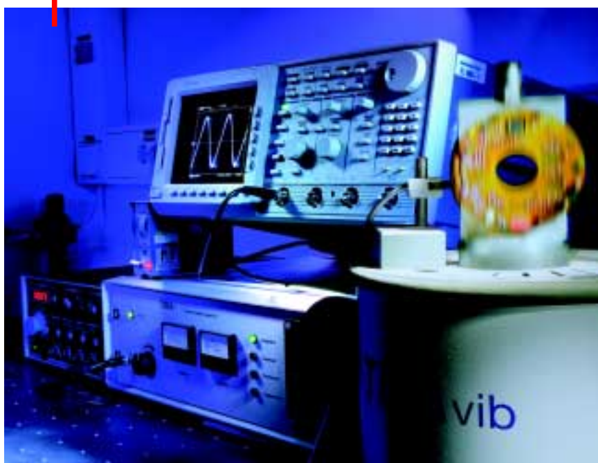
Figure 19: Vibration test, particularly with regard to resonance frequencies; the electronics board of a HeavyDuty® Digital-Tacho (encoder) for the analog-digital combination TDP 0,2 + OG 9 in the frequency range 2 Hz to 4 kHz being tested on a test bench with air suspension.
