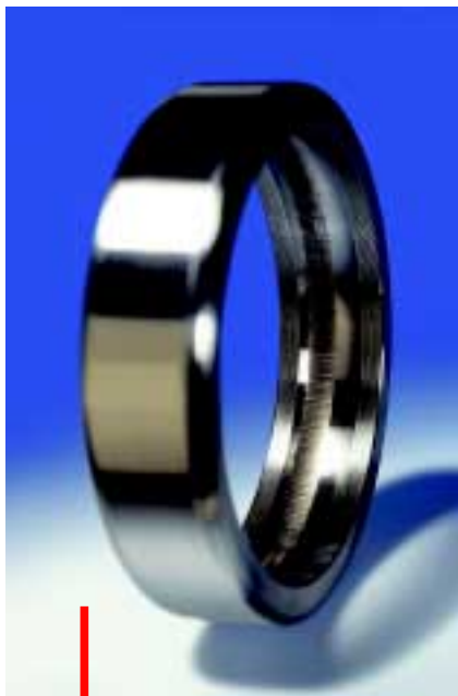
Figure 18: Ball bearings damaged by shaft currents are marked by a corrugated ball race surface.
