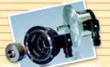
Hollow-shaft:  $\emptyset$  12; 14; 15; 16 mm Max. speed: 9,000 → 6,100 rpm Moment of inertia: 0.4; 0.6 kgcm<sup>2</sup> Weight rotor: approx. 110; 160 g Housing:  $\emptyset$  70 mm Protection: IP 55
